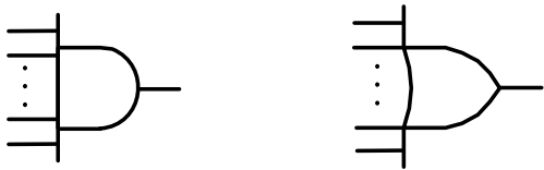
Figure 3.3 Multi-input AND and OR Logic Gates
