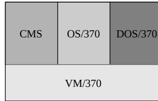
Figure 4.5 Virtual machine operating system VM/370.
